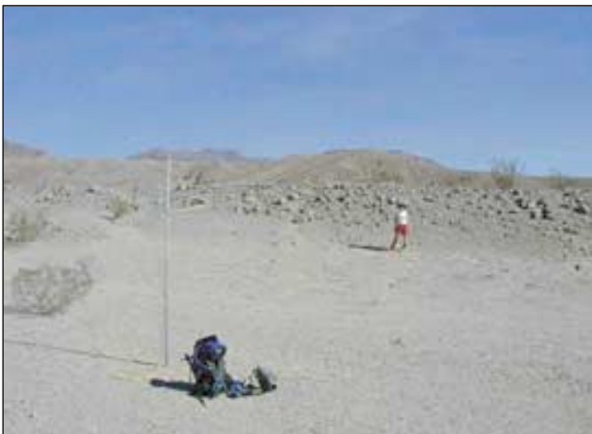
Figure M-4. Scarp profile setup. Steel measuring tape strung across two vertical rods.
